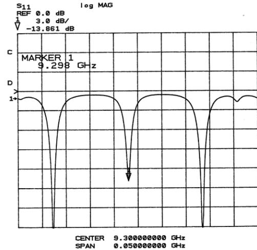
Figure 3: Extended 6-MeV Linac Stop Band.
