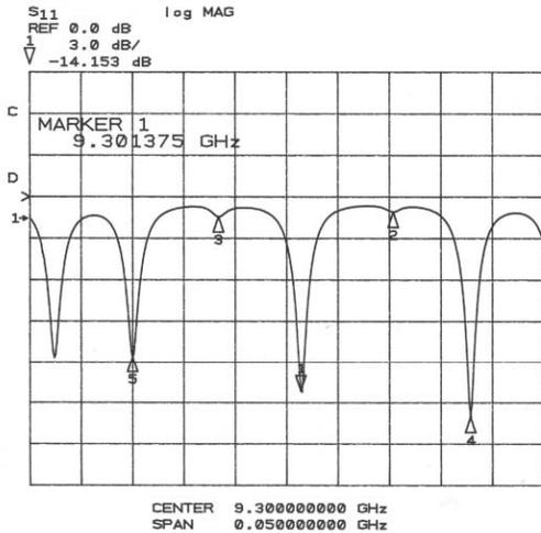
Figure 1: MINAC-6 Linac Stop Band.
