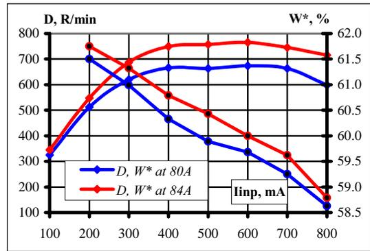
Figure 4: Extended 6-MeV accelerating system prototype output characteristics.
