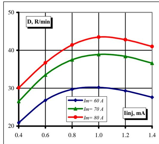
Figure 6: Dose at 1 m and 100 pps (50% of nominal RF power) versus input current for MINAC-1.
