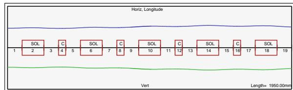
Figure 4: 500 mA 20 MeV Ne<sup>1+</sup> Beam in 15 T, 15 cm solenoid lattice separated by 25 cm including accelerating cavities.
