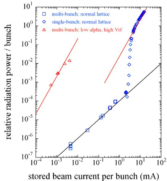
Figure 4; CSR power vs. stored current per bunch. (square: normal  $\alpha$  with multi-bunch, diamond: normal  $\alpha$  with single bunch, triangle: low  $\alpha$  with multi-bunch)
