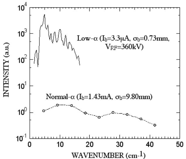
Figure 5; CSR power spectrum in the normal and the low  $\alpha$  modes.
