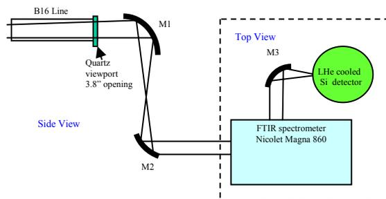
Figure 4: CSR power and spectrum measurement.
