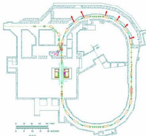
Figure 2: SHR ring plan view. Red arrows: IR beam line locations.
