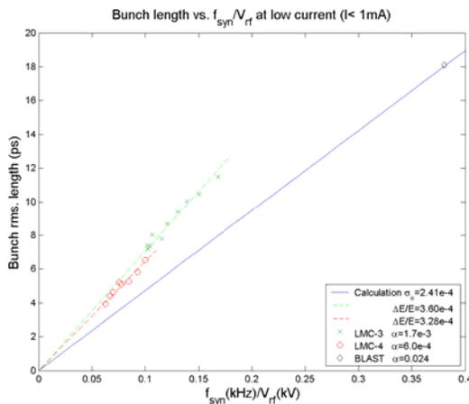
Figure 3: Bunch length vs.  $f_{\text{syn}}/V_{\text{rf}}$ .
