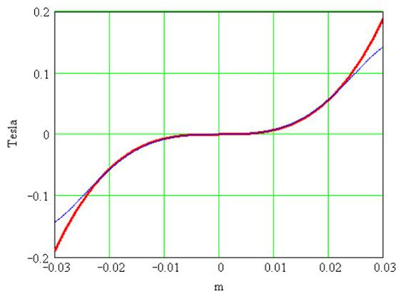
Figure 5: Octupole configuration  $\frac{\partial^3 B}{\partial x^3} = 42000 \cdot \frac{\text{Tesla}}{m^3}$
