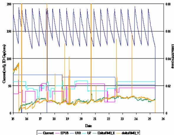
Figure 6: Rms orbit errors over a user run.
