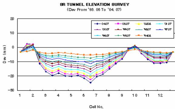
**Figure 1: Settlement of the storage ring floor since 1993 (From '93. 06 to '04. 07).**
