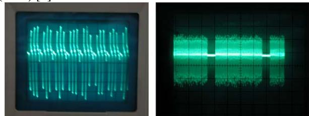
Figure 2: Filling pattern 1110-mode in the storage ring.
