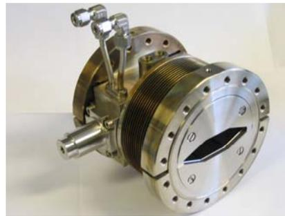
Figure 1: The first of series of BPM-bellows module
