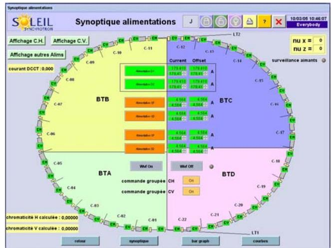
Figure 8: Screen shot of power supplies GlobalScreen driving application
