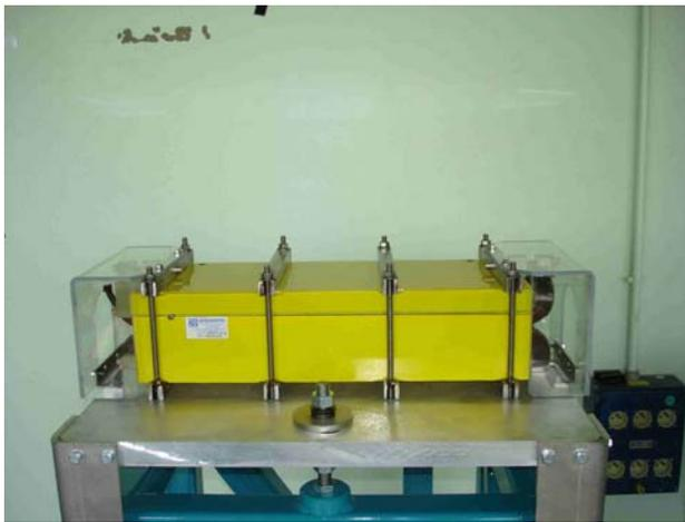
Figure 5: Booster bumper magnet.
