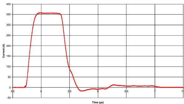
Figure 6: Measured current in the booster kicker magnet.
