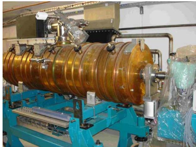
Figure 4: RF cavity in the tunnel.
