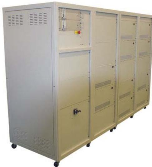
Figure 2: Picture of the pulsed dipole power supply (3 Hz, 1 kV, 0.5 kA).
