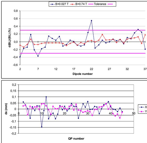
Figure 1: Dipole relative magnetic length spread (up) and quadrupoles magnetic center spread (down).
