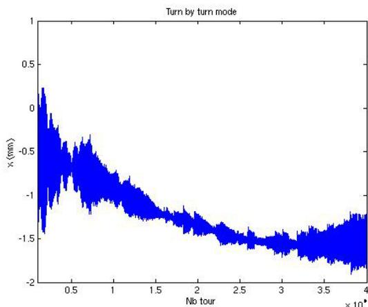
Figure 7: ESRF booster turn by turn orbit recorded with the SOLEIL Libera electronics
