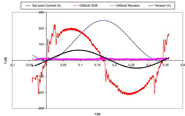
Figure 3: Systematic and random current shift on the 3Hz power supplies.
