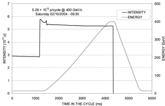
Figure 2: Beam transmission in the SPS at the end of the run. Transition crossing at  $\gamma_t = 22.8$ ,  $t=1485$  ms.
