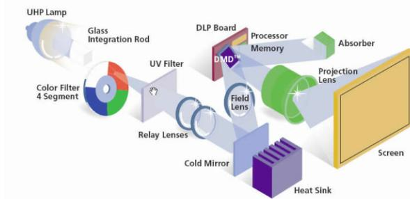
Figure 8: Display Wall projection engine.
