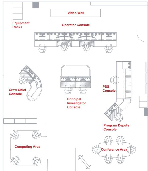
Figure 7: New control room layout.
