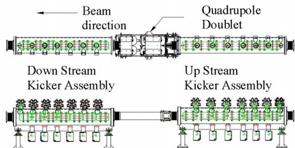
Figure 3. SNS extraction fast kicker magnet arrangement
