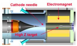
Figure 6: Immersed B Field Diode
