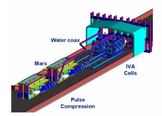
Figure 8: The two CYGNUS IVAs as configured at the NTS.
