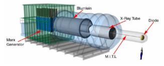
Figure 2: The Single (Blumlein) Pulse Forming Line Pulsed Power Machine.
