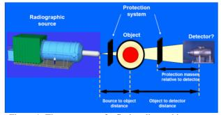
Figure 1: The geometry of a flash radiographic system.
