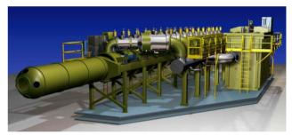
Figure 9: The 10 stage IVA for new AWE radiographic facilities.
