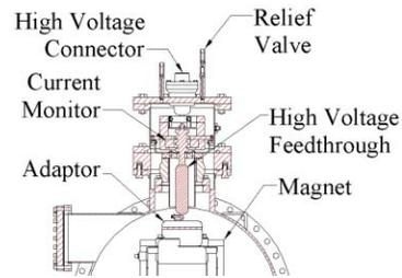
Figure 4: High Voltage connection.
