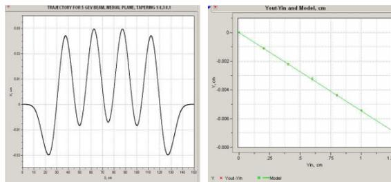
Figure 6: Trajectory of electron with energy 5 GeV entering at  $x=y=0$ , left. Difference between exit and entrance  $y$ -coordinates and the linear model fit, right.
