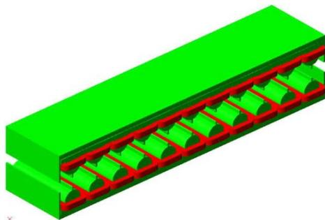
Figure 3: Wiggler with profiled poles.
