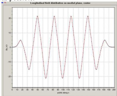
Figure 5: Longitudinal field dependence (as function of  $s$ ) at  $x=0$  calculated for wiggler Fig. 3 with tapering  $\sim 1/4, 3/4, 1$ . Right point on this picture corresponds to  $s=150$  cm.
