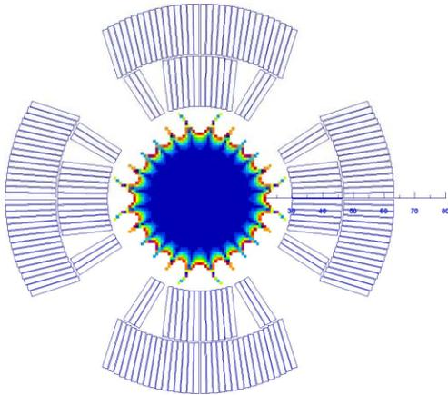
Figure 4. Coil cross-section of a 60 mm aperture quadrupole using 16.4 mm Nb<sub>3</sub>Sn cable.
