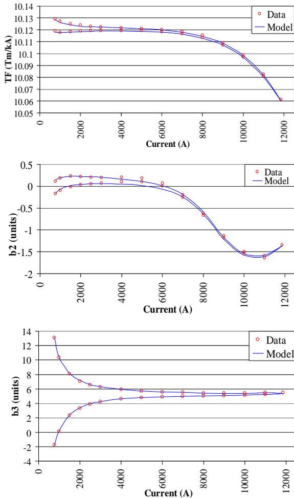
Figure 1: Modeling of the transfer function (above), the normal dipole (center) and the normal sextupole (below) for a loadline cycle.
