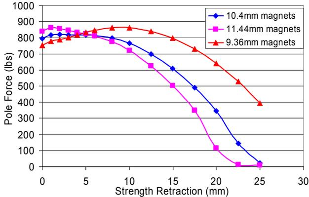
Figure 4: Pole force for three magnet thicknesses vs. Strength Retraction.
