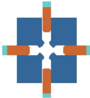
Figure 1: Method of achieving strength adjustment by uniformly retracting all four magnets in a PM Quad.
