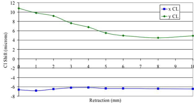
Figure 8: Magnet angle sensitivity. Angle of one magnet was changed by 5 degrees. Sensitivity is approximately 1 micron/degree.
