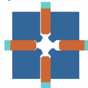
Figure 2: Method of shifting the horizontal magnetic centerline to the right by shifting a pair of magnets. (Highly exaggerated for illustration purposes.)
