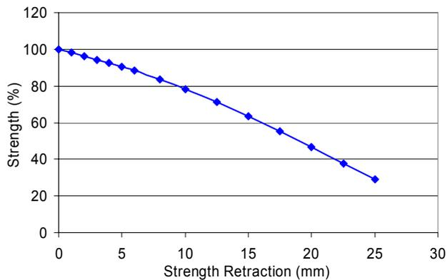
Figure 5: Strength tuning curve for 10.4mm thick magnets, 13mm aperture, 1.03T pole tip field.
