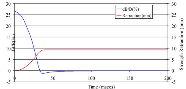
Figure 9: Eddy Current analysis of peak field change vs. time (dB/B) for a rapid field adjustment.
