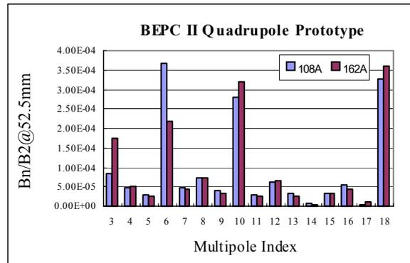
Figure 5: Multipole error spectrum for BEPCII quadrupole prototype.
