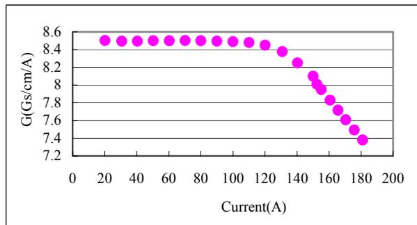
Figure 3: Transfer function of quadrupole magnet prototype.
