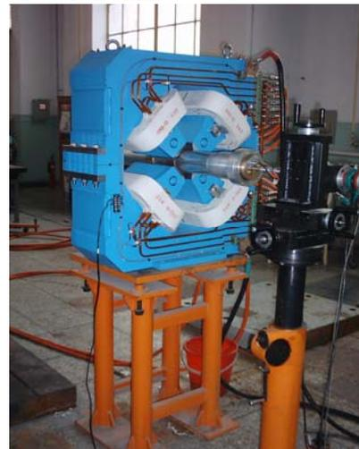
Figure 1: Field harmonics measurement system of BEPCII quadrupole magnets.
