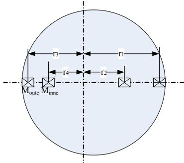
Figure 2: The pick-up coil cross section.
