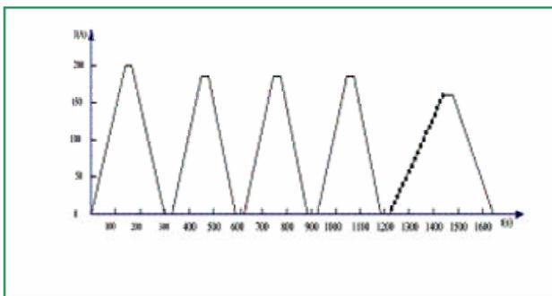
Figure 4: Pre-cycle and ramping cycle for BEPCII quadrupole magnets.
