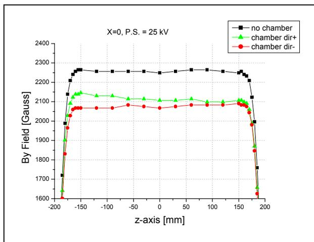
Figure 3: Zooming the plateau of the field measurement on the centerline along electron beam direction.
