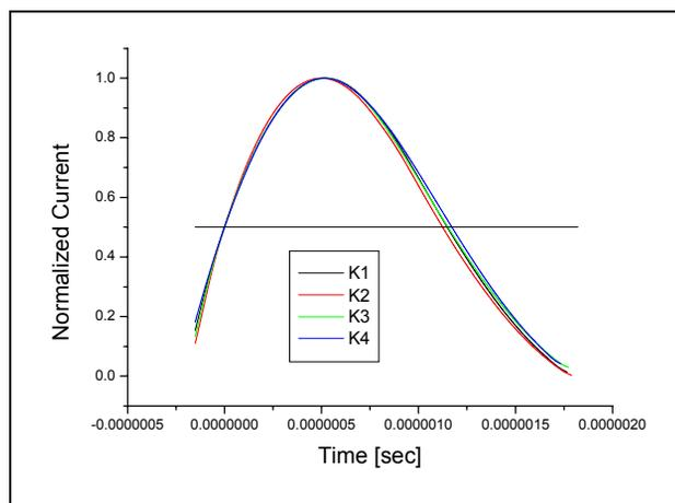
Figure 4: Mismatch of four kicker waveform.
