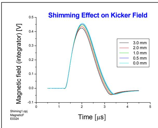
Figure 6: The shimming effect on the change of magnetic field waveform.
