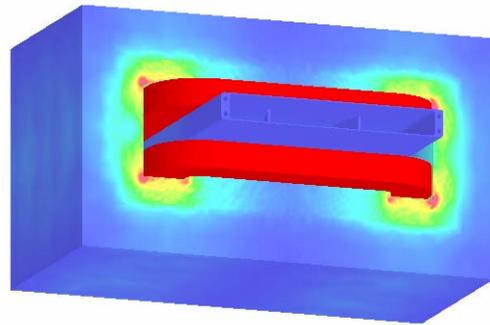
Figure 6: Surface contours of magnetic field by ELEKTRA code.
