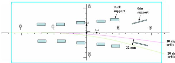
Figure 4: Supports in vacuum chamber with orbits of 10 and 20 degree deflections.
