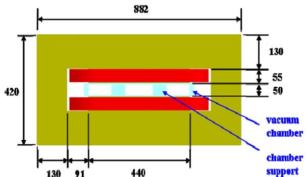
Figure 3: Iron core size with vacuum chamber.
