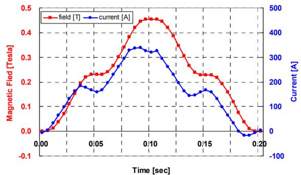
Figure 7: Calculated current and magnetic field for half period.
