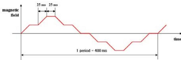
Figure 2: Required magnetic field waveform.
