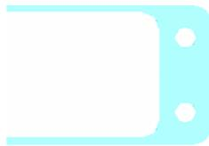
Figure 5: Cross section of the cooling channels at the corners of vacuum chamber.
