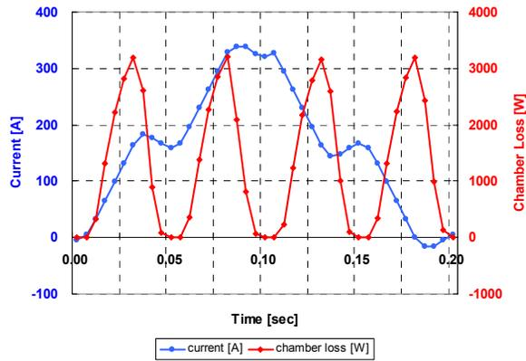
Figure 8: Currents and vacuum chamber losses for half period.
