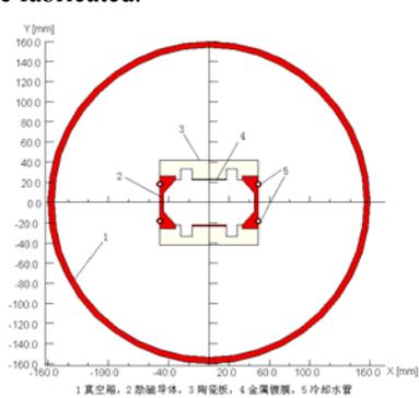
Fig.6 Layout of injection kickers for the BEPCII storage rings
