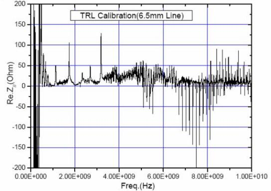
Fig.3 Impedance of the bellows without RF rings shielding (using TRL calibration technique)
