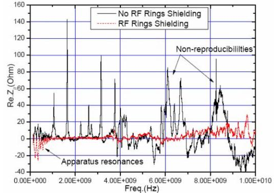
Fig.4 Impedance of the bellows without RF rings shielding (using reference pipe and absorbers)
