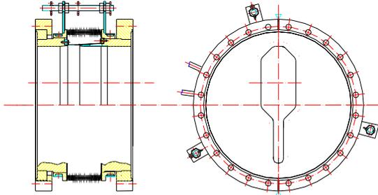
Fig.2 RF-shielded bellows for the BEPCII
