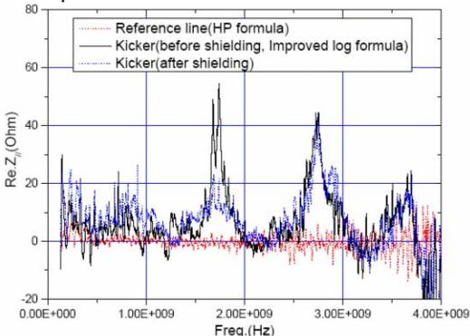
Fig.8 Impedance of the injection kicker for the BEPCII
