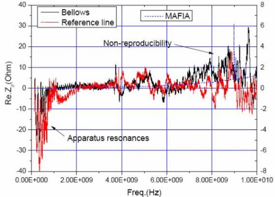
Fig.5 Impedance of the bellows with RF rings shielding (using reference pipe and absorbers), comparing with that of reference pipe
