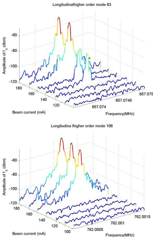
Figure 2: The dependence of the amplitude of synchrotron sideband on the total beam current. The top graph is the measurement for the longitudinal mode at 657 MHz, and the bottom is for the mode at 762 MHz. The threshold current is 130 mA for the longitudinal mode at 657 MHz and 140 mA for the mode at 762 MHz respectively.
