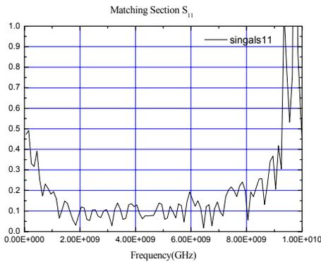
Figure 3: performance of the gradual change impedance matching section
