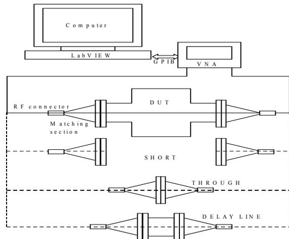
Figure 6: TRL based longitudinal impedance measurement
