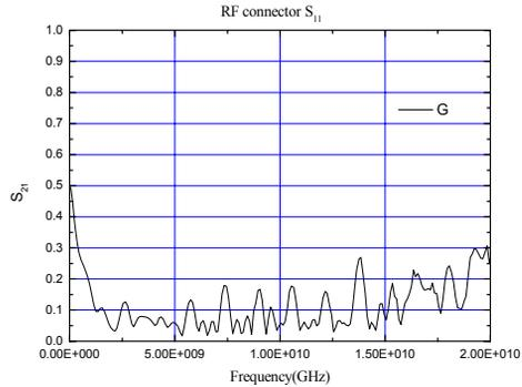
Figure 5: S<sub>21</sub> of the special designed RF connector
