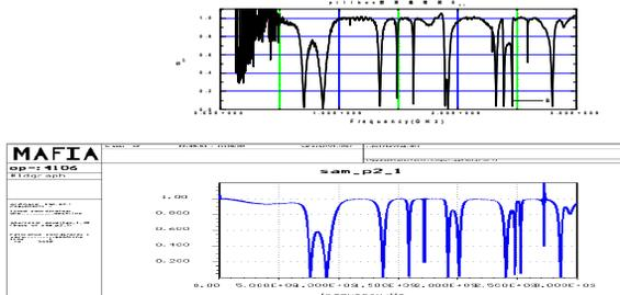
Figure 8: Measured and calculated  $S_{21}$  of the pillbox
