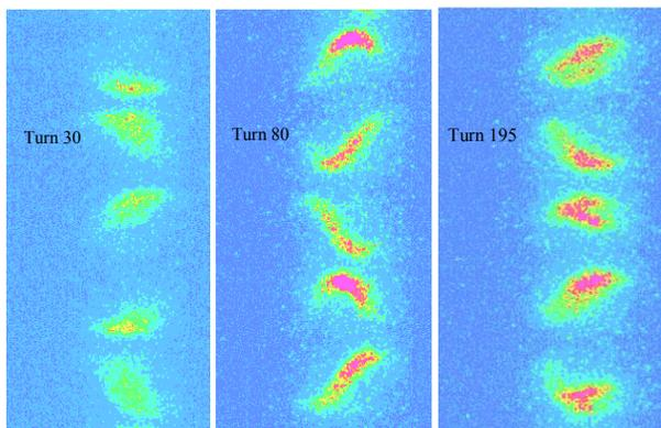
Figure 7: Side-view streak images of 0.2 mA bunches with turn indices (left) No. 29 to 33, (middle) No. 89 to 93, and (right) No. 194 to 198.
