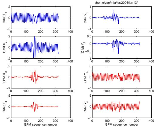
Figure 1: *Four independent orbits extracted from PEP-II LER BPM buffer data taken on January 13, 2004. The first two orbits ( $x_1, y_1$ ) and ( $x_2, y_2$ ) are extracted from beam orbit excitation at the horizontal tune while the other two orbits ( $x_3, y_3$ ) and ( $x_4, y_4$ ) are from excitation at the vertical tune.*
