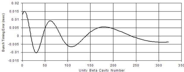
Figure 4: Propagation of SNS level phase and energy jitter from 1.2 to 8 GeV leading to maximal output phase error.
