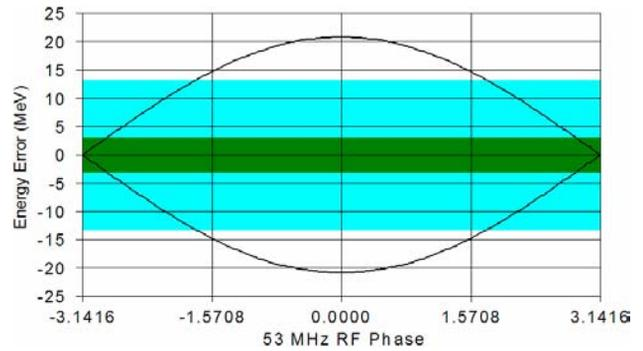
Figure 12: The dark (green) shaded area is the output 95% energy spread of the Proton Driver when only a debuncher cavity is used.
