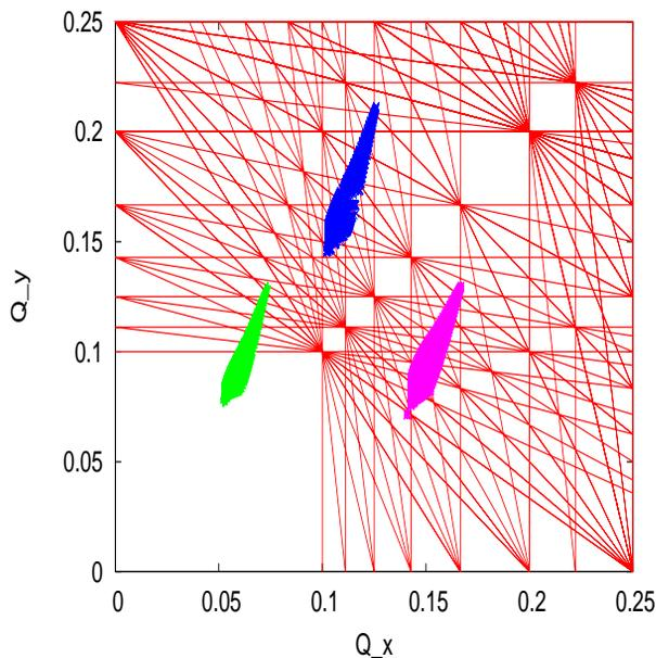
Figure 2: Resonances up to 10th order and necktie diagrams for the three possible eRHIC working points investigated in this study.
