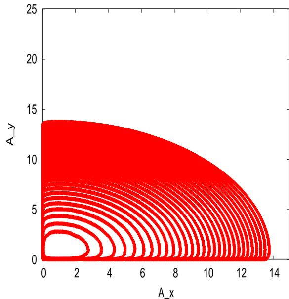
Figure 3: Density contours in the absence of the beam-beam interaction, resulting from the simulation. The density decreases by a factor 10 between level lines.
