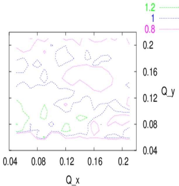
Figure 1: Contour plot of the resulting normalized luminosity  $\mathcal{L}/\mathcal{L}_0$  vs. horizontal and vertical electron beam tune.  $\mathcal{L}_0$  denotes the geometric design luminosity according to Table 1.
