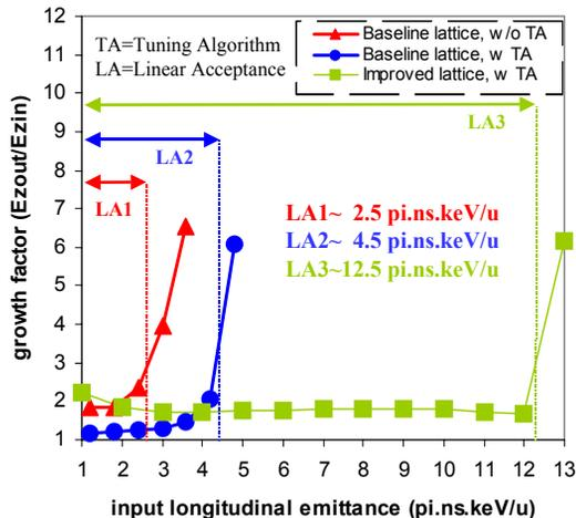
Figure 2: Longitudinal emittance growth factor for  $U^{28+,29+}$  beam in segment 1 of RIA SC linac for various input emittance values. The growth factor is the ratio output emittance over input emittance.
