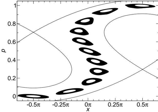
Figure 2: Phase space for the case  $a = 1/12$ ,  $b = 1/6$ , showing separatrixes (solid lines) and a bunch being accelerated from  $p = 0$  to  $p = 1$ .
