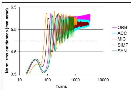
Figure 4:  $\epsilon_y$  for linearized AG lattice,  $Q_{0,x} = 6.207$ .
