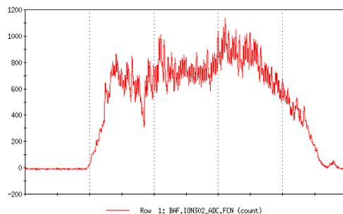
Figure 2: Normal slow extracted beam spill using rf phase displacement to smooth spill harmonics.
