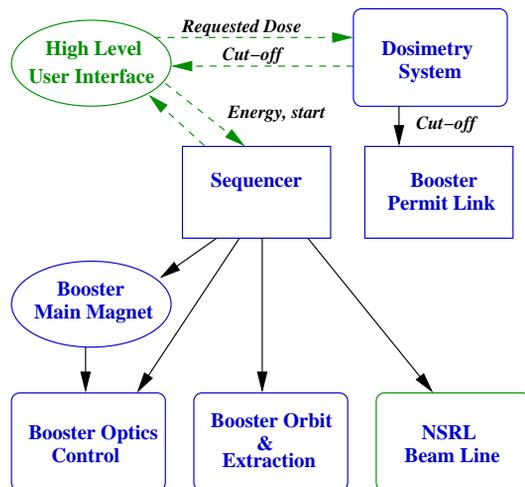
Figure 1: Solar particle simulator software system diagram.
