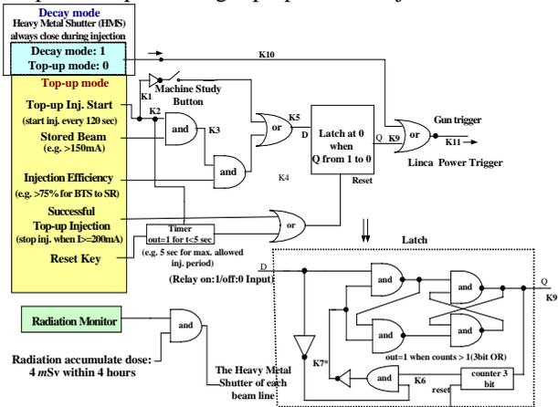
Figure 4: The logic diagram of top up mode interlock system.
