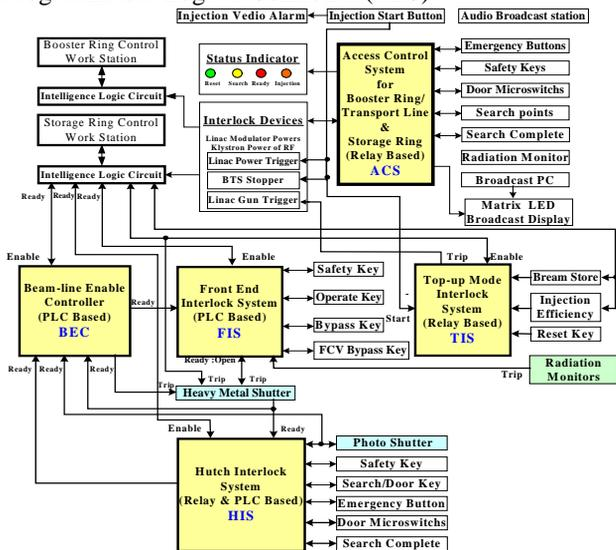
Figure 2: The main flow diagram of the safety interlock system showing the overall safety system and the related subsystems at NSRRC.
