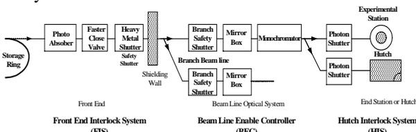
Figure 3: The layout of subsystems associated with beamline operations.
