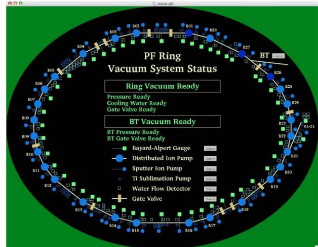
Figure 2: Monitor panel of the PF ring vacuum system status.
