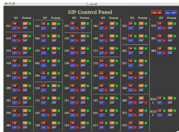
Figure 3: Control panel of the sputter ion pumps.
