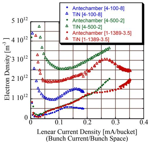
Figure 5: Electron (cloud) density in an antechamber type duct and the TiN coated chamber under various bunch patterns. The location is different. The notation of bunch pattern in the legend means [Number of train - Bunch per train - Bunch space (rf bucket as a unit)].
