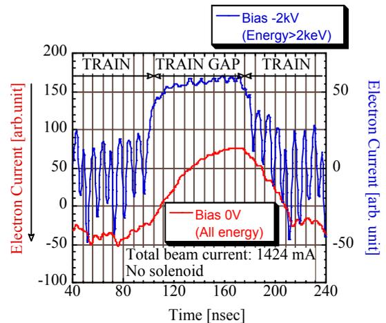
Figure 2: Time variation of the number of electrons impinging on the chamber wall by MCP.
