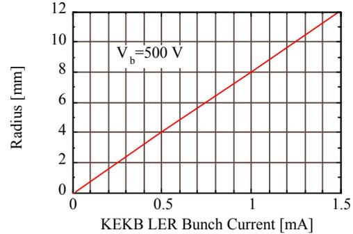
Figure 3: Radius of the observed volume.  $f_{rev}$  of KEKB LER is 9.94 kHz.
