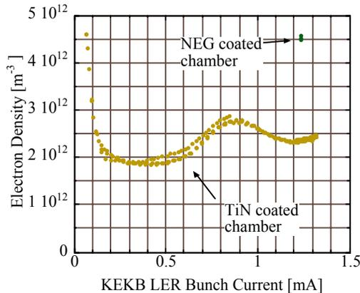
Figure 4: Electron (cloud) density in a NEG coated chamber and a TiN coated chamber. NEG coating was performed by BINP with the permission by SAES Getters and CERN. TiN coating was performed by BNL.
