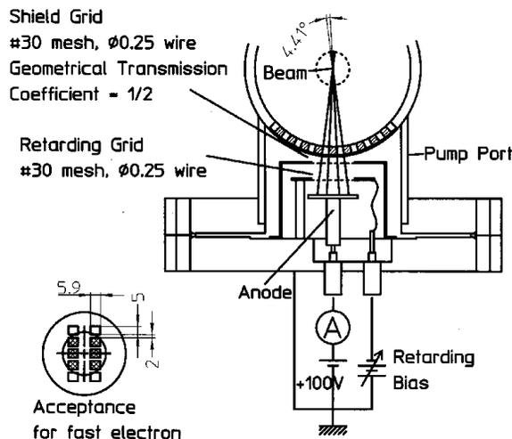
Figure 1: Schematic drawing of an RFA at a pump port of a KEKB LER duct.
