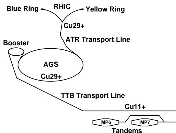
Figure 1: Acceleration of copper ions for RHIC.
