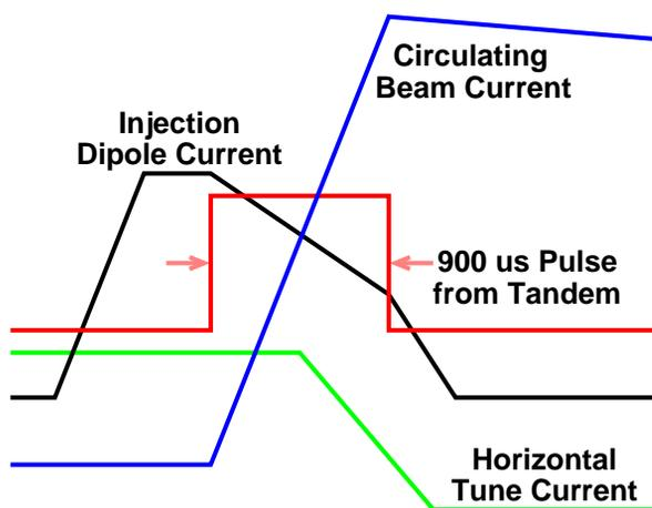
Figure 2: Typical timing at Booster injection.
