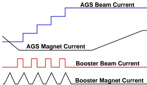
Figure 3: Timing of Booster and AGS cycles. Each Booster cycle is 200 ms long.
