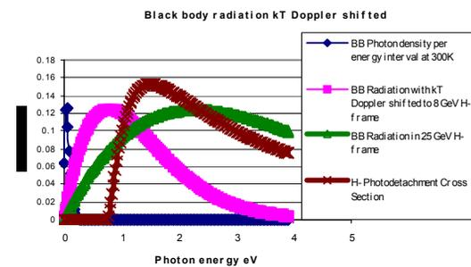
Figure 1: The brown curve is the photodetachment cross section. The Doppler effect shifts the 300 °K thermal photon distribution curve from blue (rest H<sup>-</sup>) to pink (8 GeV H<sup>-</sup>) and green (25 GeV H<sup>-</sup>) respectively. The overlapping between the photon distribution and cross section curves gives rise to blackbody radiation stripping.
