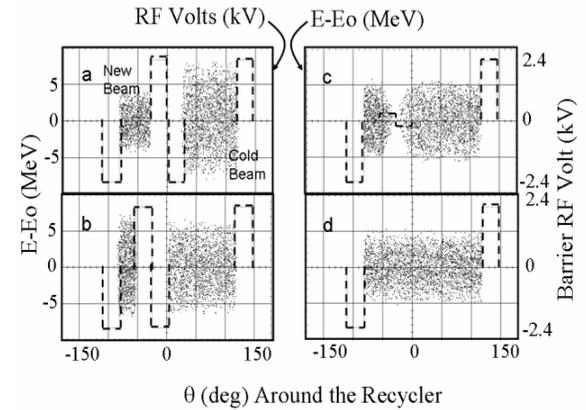
Figure 3: ESME simulations for proposed scheme a) two stacks of beam with different energy spreads,  $\pm 4.4$  MeV (new beam) and  $\pm 8.2$  MeV for (cold beam). In the present case the new and cold beams are just symbolic
