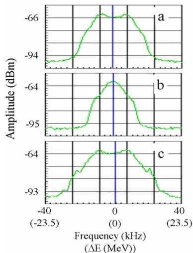
Figure 4. Schottky data for beam in barrier buckets of a)  $T_A=2.7 \mu$ s, rms  $\sigma_A=4.1$  MeV,  $\epsilon_A=48$  eVs b)  $T_B=1.59 \mu$ s, rms  $\sigma_B=2.2$  MeV  $\epsilon_B=14$  eVs, (before energy matching and merging,) and c)  $T_{final}=3.27 \mu$ s, rms  $\sigma=4.8$  MeV,  $\epsilon_A=68$  eVs(after merging using proposed scheme).
