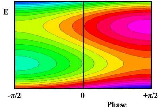
Figure 6: Serpentine acceleration path (yellow) in longitudinal phase space for linear non-scaling FFAG.
