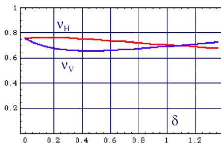
Figure 8: Tune variation with momentum for an AFP FFAG replacement of the 1.5 GeV AGS Booster.
