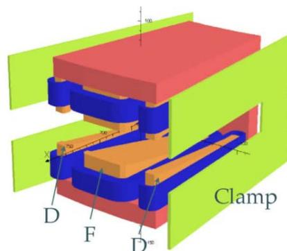
Figure 3: Magnet for the PRISM muon phase space rotator.
