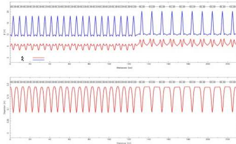
Fig. 7: Lattice function matching between normal cells and insertion cells in an isochronous FFAG at 14.75 GeV.
