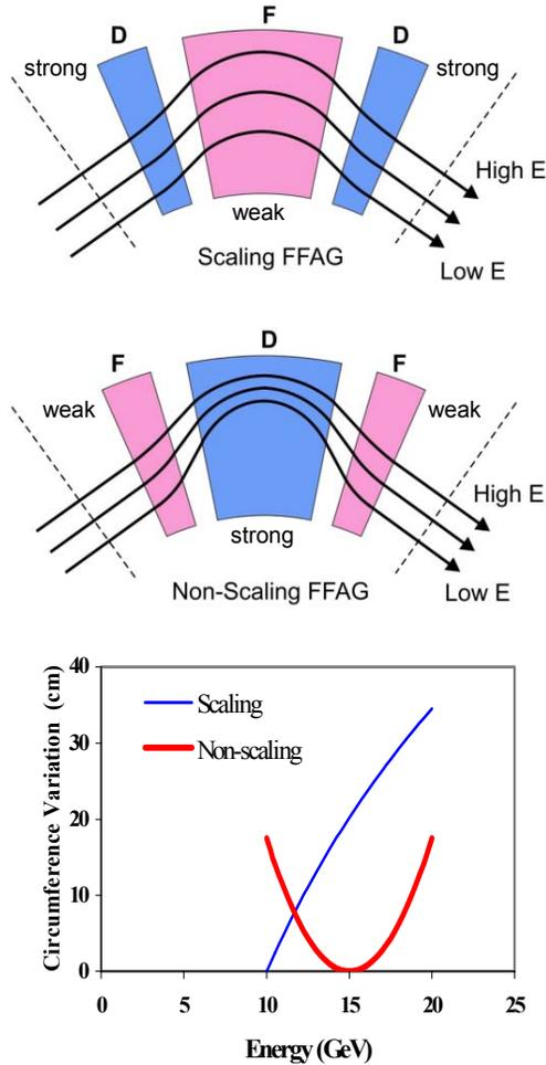
Figure 5: Scaling and non-scaling FFAG orbit patterns (above), and circumference variation with energy (below).
