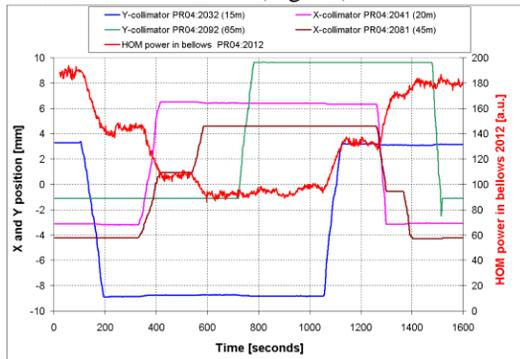
Figure 11: HOM power (red line) in the arc bellows and beam position near vertical (blue and green lines) and horizontal collimators (pink and brown lines).
