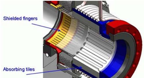
Figure 14: Straight section HOM absorber
