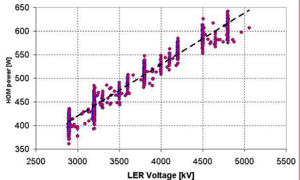
Figure 9: HOM power as a function of RF voltage for a positron current of 1400 mA.
