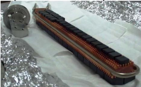
Figure 6: Water-cooled HOM absorber.
