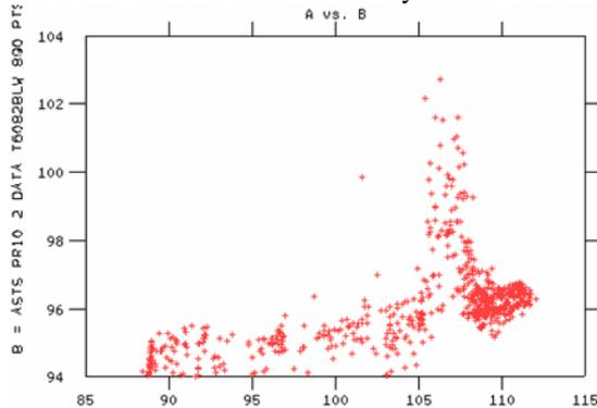
Figure 17: Bellows temperature (°F) as a function of vacuum chamber temperature (°F).
