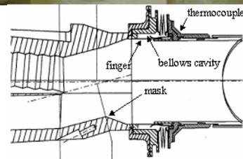
Figure 4: Vertex bellows structure and vacuum chamber showing synchrotron masks and site of thermocouple with high temperature readings.
