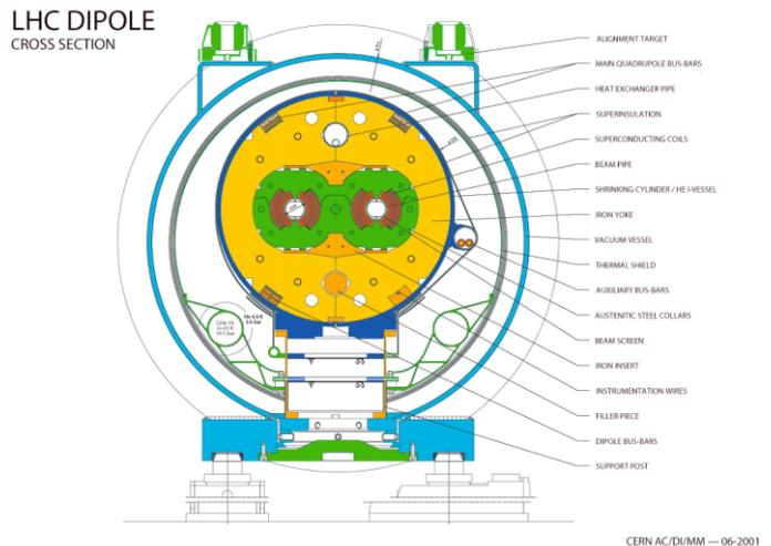
Fig. 1. Cross section of the LHC Main Dipole in its cryostat.
