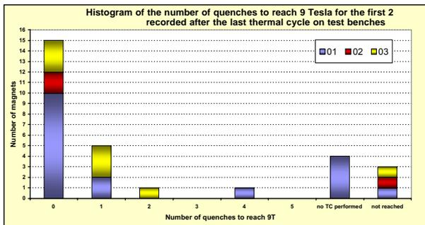
Fig. 3 Number of quench for each of the 29 dipoles tested so far, after first thermal cycles to reach ultimate field of 9 T.
