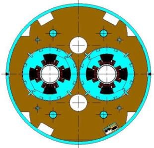
Fig. 2. Cross section of a MQY, with its very thin iron among the apertures
