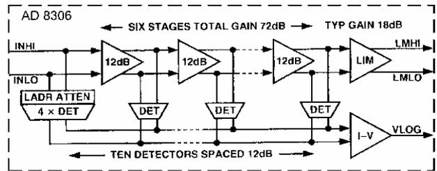
Fig. 5. Functional block diagram of the AD8306 log amplifier (source Analog Devices).
