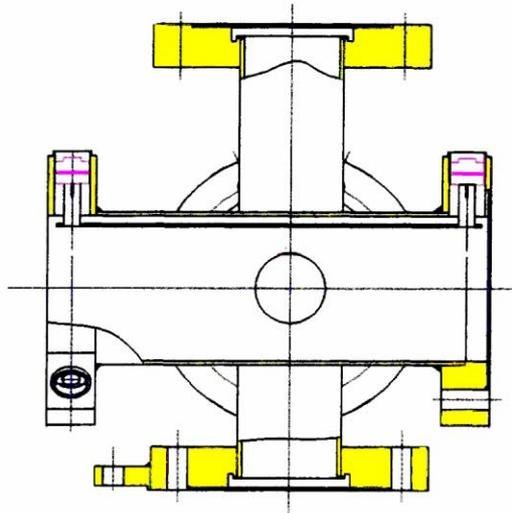
Fig. 2. Longitudinal view, showing the stripline ports.
