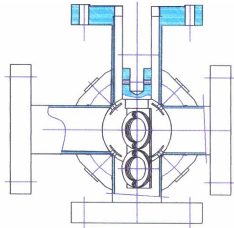
Fig. 1. Schematic drawing of the new diagnostic station combining two screens (OTR and scintillator) and a 4-stripline BPM : transverse view, showing the screens.
