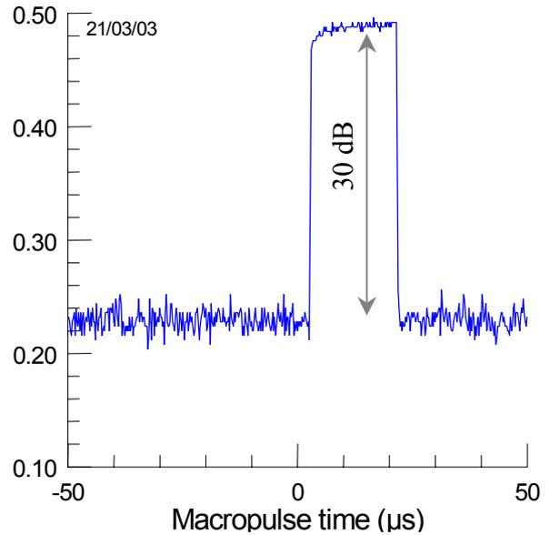
Fig. 8. Response of a  $\Sigma$  channel, on ELSA. The macropulse is 20  $\mu$ s long. Vertical scale is in Volts, 10 mV/dB (half the value of the AD8306 slope, because of the 50  $\Omega$  termination on scope).
