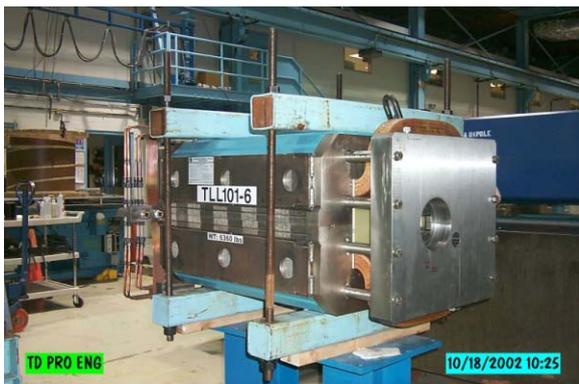
Figure 3: *Shield plate at the non lead-end extremity.*
