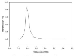
Frequency Characteristics of Etched Steel/Fluorogold Filter
