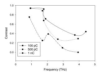
Figure 5: Degree of electron beam modulation as a function of charge and frequency.
