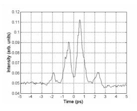
Figure 1: Cross-correlation measurement of 266-nm drive laser pulse incident on photocathode (Head of pulse on right).
