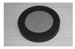
Figure 3: Etched steel terahertz filter.
