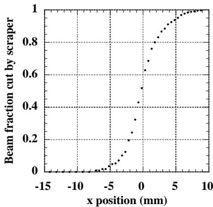
Figure 3: Measured beam fraction cut by the scraper as a function of the scraper position. The beam current was 5 mA. A symmetric transverse profile was assumed in data processing.
