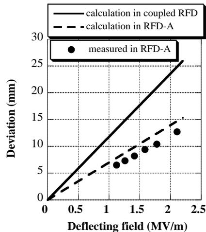
Figure 5: Measured deflecting beam position at the scraper in the single RFD-A system vs. deflecting field of the RFD. The calculated deviation for both the RFD-A and the coupled system are also plotted.
