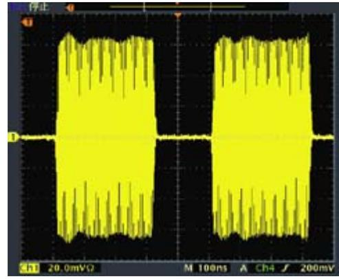
Figure 7: Signal of a chopped beam measured by the eighth BPM. The beam current is 24 mA.  $P_{in}=36$  kW. The phase-reversal switch was turned on. 100 ns/div.
