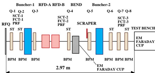
Figure 1: Layout of the MEBT.
