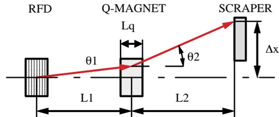
Figure 4: Deflecting scheme of a single RFD system.
