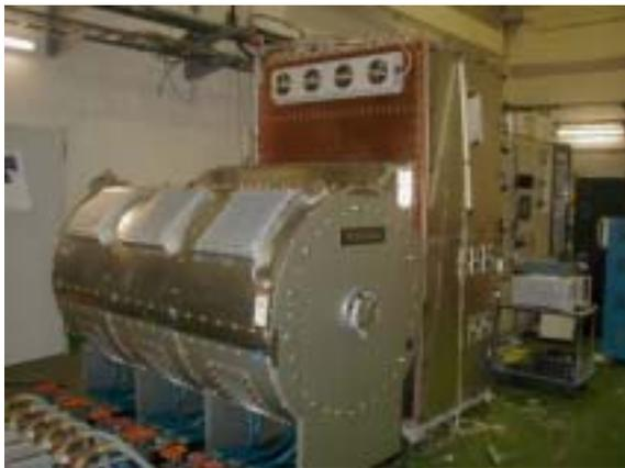
Figure 7: The RF cavity for the MR
