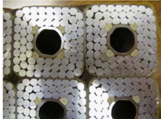
Figure 5: The stranded conductors impregnated by the polyimide resin to form the coil
