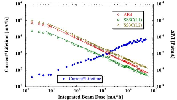
Figure 2:  $I\tau$  and  $\Delta P/I$  versus the integrated beam dose.
