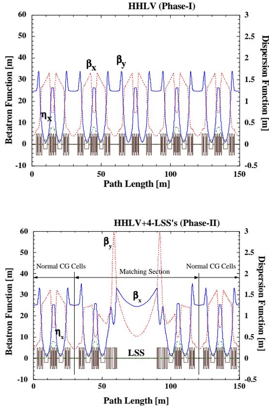
Figure 1: Phase-I and Phase-II optics.
