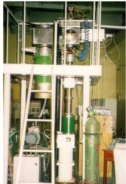
Figure 2: The test stand of the H- ion source and axial injection line.
