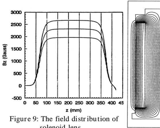
Figure 9: The field distribution of solenoid lens.
