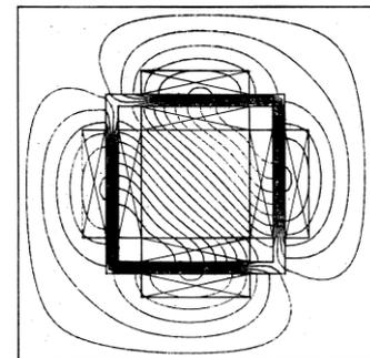
Figure 8: The field distribution of x-y steering magnet.
