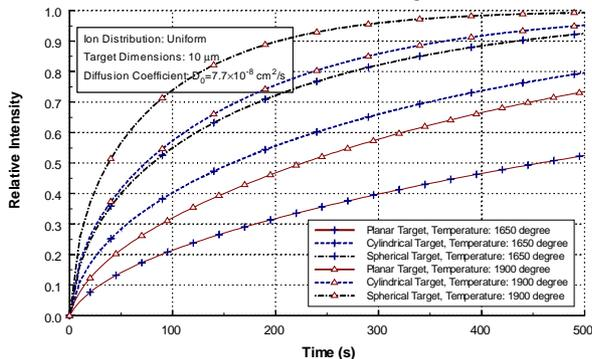
Figure 10: The release time of  $^{19}\text{F}$  diffusing from  $\text{ZrO}_2$  at different operation temperature.
