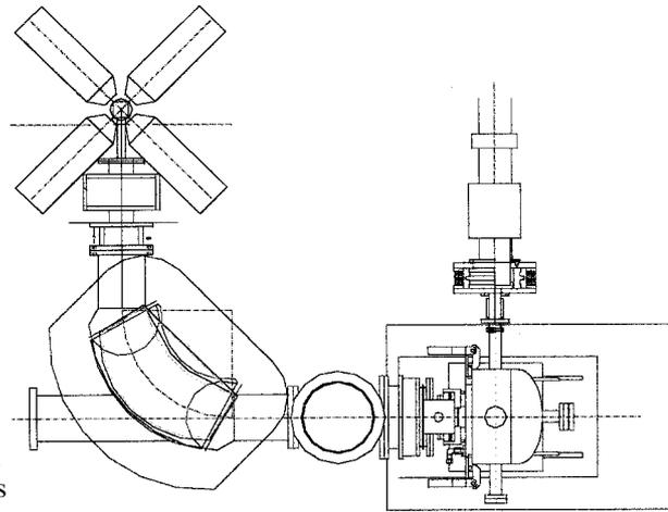
Figure 11: The ISOL test system used for the keV RIB generation.
