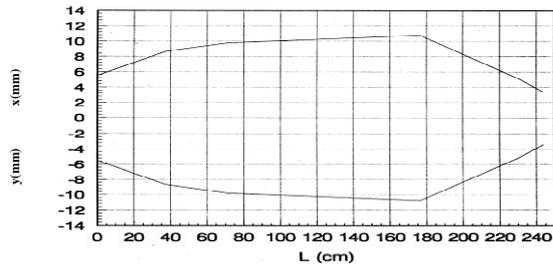
Figure 7: The envelope of the axial injection line.
