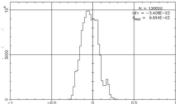
Figure 4: Azimuthal projection of rotated bunch shown in Fig. 3, abscissa in degrees. The rms bunch length in time is 0.64 ns.
