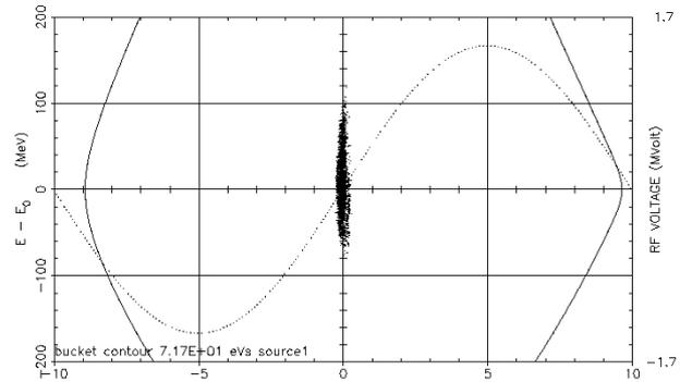
Figure 3: Energy [MeV] vs. azimuth [deg] distribution of .43 eVs bunch of  $1.7 \cdot 10^{12}$  protons at 16 GeV after quarter period rotation at 1.4 MV, Stage 2 Proton Driver.
