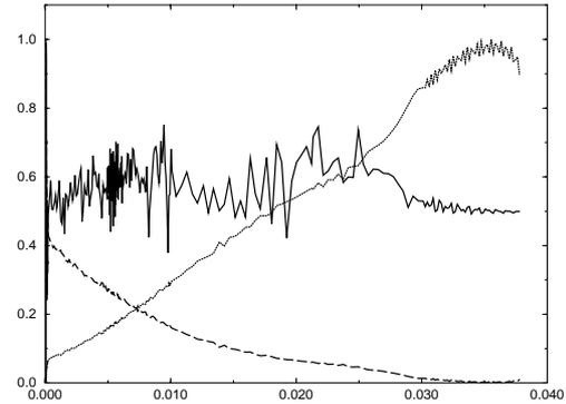
Figure 2: RMS normalized emittance (solid), rms bunch width (dashes), and rms bunch height (fine dots) for the stage one acceleration cycle, all scaled to plot in the range 0 to 1.
