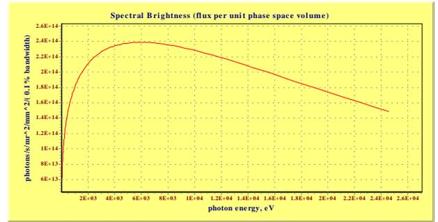
Figure 4: Spectral brightness of 1mr of arc in horizontal plane.
