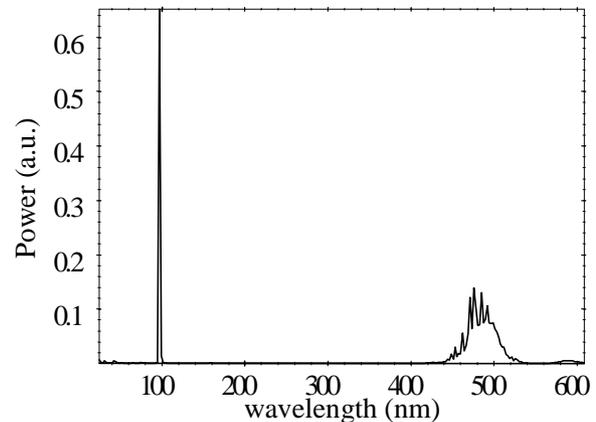
**Figure 4:** The same electron bunch as in fig.3 but with a seed laser, at  $\lambda_r$ . The enhancement of the 5<sup>th</sup> harmonic is 5 times bigger than without seed laser.
