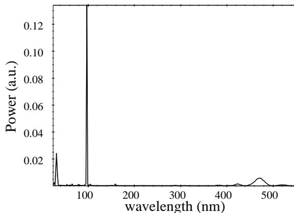
**Figure 3:** Same electron bunch as in fig. 2, at the end of the radiator. The 5<sup>th</sup> harmonic is enhanced.
