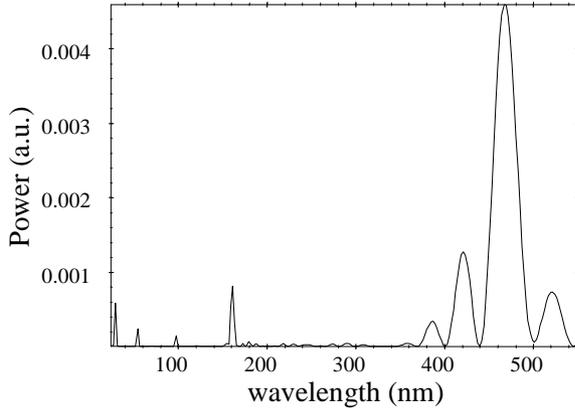
**Figure 2:** Spectral power from a 100 fs electron bunch at 100 MeV and 0.1 nC, crossing an undulator of 10 periods 25 mm length,  $K=1$ .
